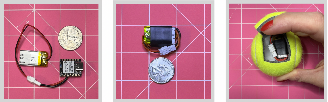
Figure 2: Left panel shows the battery and microcontroller with a quarter for size reference. Middle panel shows the battery and microcontroller wrapped into a module. The right panel shows the module embedded into a ball. Here, you can also see the opening that was cut into the ball.
